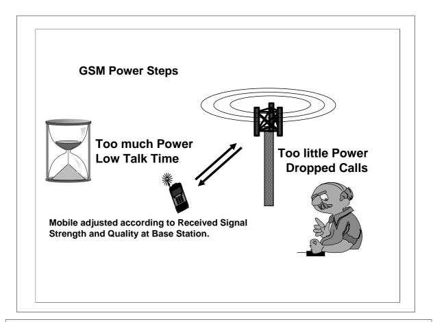
As the mobile moves around the cell, its transmitter power needs to be varied. When it's close to the base station, power levels are set low to reduce the interference to other users. When the mobile is further from the base station, its power level needs to increase to overcome the increased path loss. However, if too much power is used, the user's battery will run down too quickly.
