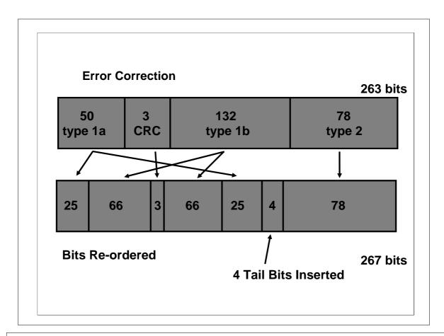
The next step is to 'shuffle' the bits around so that they are no longer in sequential order. This means that when they are transmitted, the loss of one section can still be rectified using the error correction schemes (described next) and the fact that not all bits have been lost.
