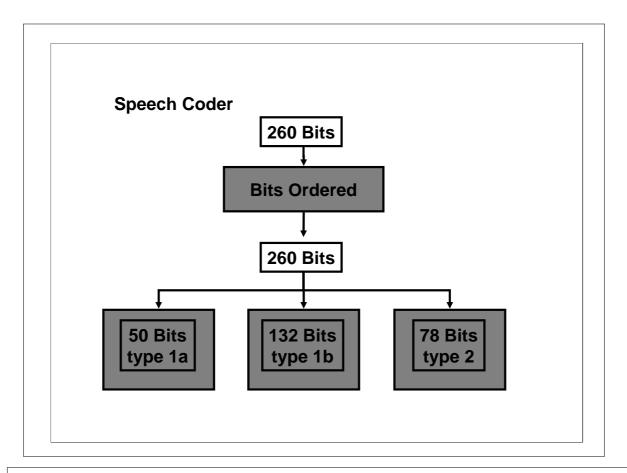
Now that the voice has been modeled, it needs to be protected on its rough journey through the hostile Rf environment. The vocoder will output 260 bits of three types or classes 1a, 1b and 2(II). These are the result of the coding schemes that give rise to important, less important and unimportant bits. The point here is that they will receive different amounts of error protection in the codec.
