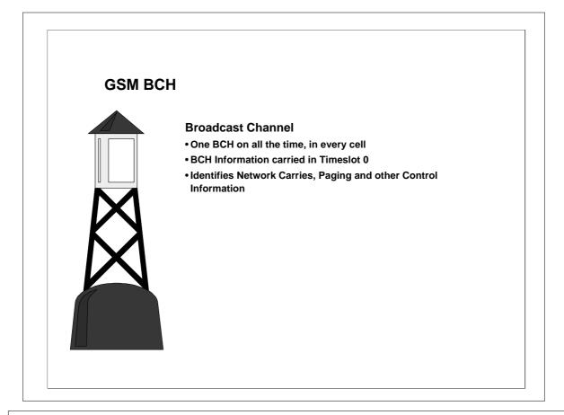
The concept of a Broadcast Channel (BCH) is very simple; the BCH acts like a beacon, or lighthouse. It's on all the time and is the first thing the mobile looks for when it's trying to find service. The BCH ARFCN has to be active in all timeslots to allow mobiles synchronized to other cells to measure its power. The useful BCH information is always carried in timeslot 0. The other timeslots are filled with dummy bursts, or are available for TCH.
