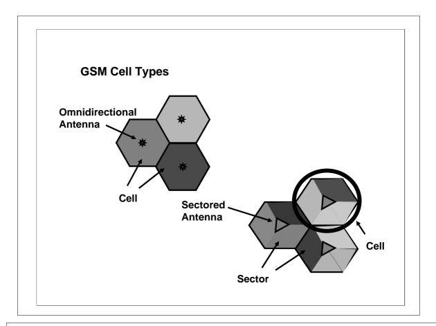
One way for cells to be designed is using an omnidirectional antenna at the center. The whole cell uses the same channels.
