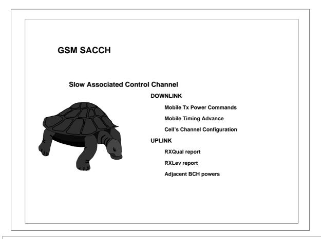
The Downlink Slow Associated Control Channel (SACCH) is used to send slowly but regularly changing control information to the mobile. Examples are instructing the mobile to change its transmitter power (MS\_Tx\_Lev) and burst timing advance (to compensate for RF transit time) as it moves around the cell.
