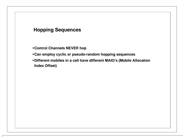
There are a few things to know about hopping cells. The BCH never hops. As the hopping process is a highly synchronized operation, and the mobiles that are not camped to the system are not synchronized, we would end up with a catch 22 situation. The mobile cannot hop because it is not synchronized, it is not synchronized because it is not camped, it cannot camp because it is not synchronized and it cannot synchronize because it cannot hop!
