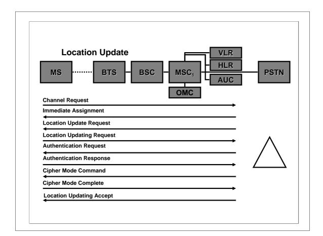
This is a step by step process for Location Updates; this time showing which part of the network is involved in transactions.
