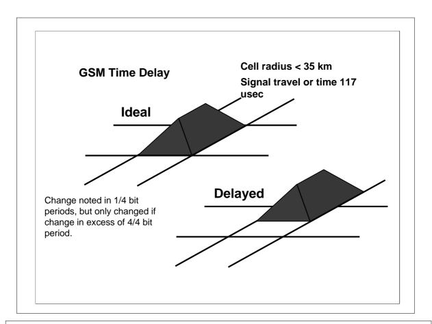
In GSM, because it uses TDMA with cells up to 35 km radius, a radio signal will take a finite period of time to travel from the mobile to the basestation. There must be some way to make sure the signal arrives at the base-station at the correct time.
