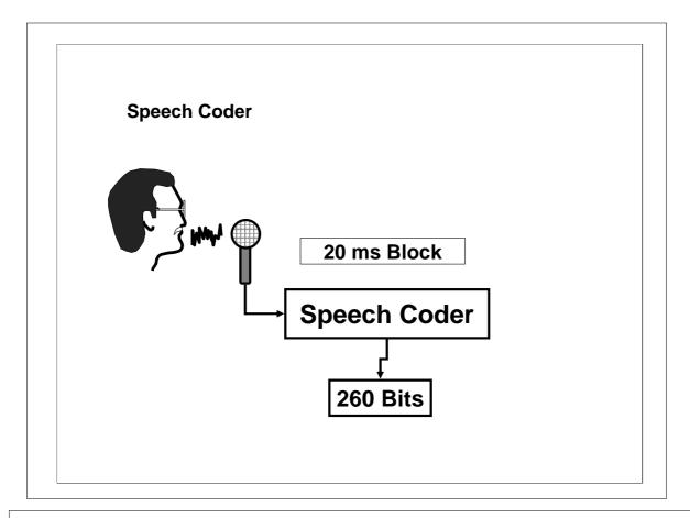
Most modern digital communications systems use some sort of voice compression. GSM is no exception. It uses a voice coder to model the tone and noise generation in the human throat and the acoustic filtering of the mouth and tongue. These characteristics are used to produce coefficients that are sent via the TCH.
