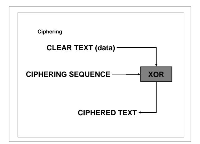
There is also a way of further scrambling the data known as ciphering. The cipher is a code that requires an intimate piece of information to be known by both sending and receiving parties. In this case it is the cipher key Ki.
