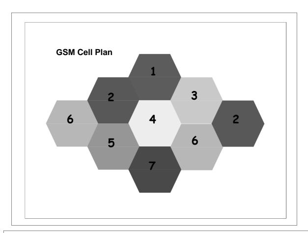
GSM uses a number of channels in each cell. However, the same channels cannot be used in adjacent cells, as they would interfere with one another. This is Spatial Division Multiple Access (SDMA), a scheme that reuses the channels in distant geographical areas.
