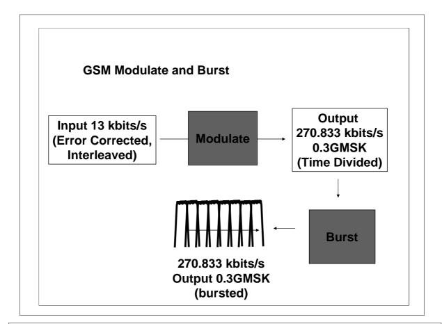
Just before modulation, one more step has to be performed. This is burst building. This is where the data blocks are added to the tail bits, stealing flags and midamble to make up the burst structure that we saw earlier. Some call this channel coding.
