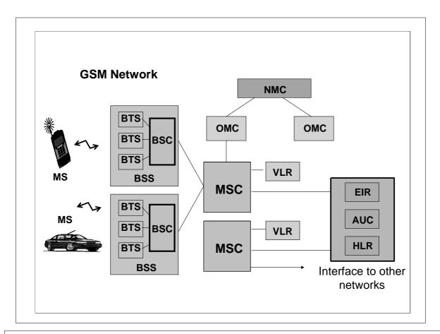
This is a simple representation of a GSM system. The Mobile Stations (MS) talk to the Base Station System (BSS) over the RF air interface. The Base Station System (BSS) consists of a Base Transceiver Station (BTS), and a Base Station Controller (BSC). It's typical for several BTS to be located at the same site, producing 2 to 4 sectored cells around a common antenna tower. BSC's are often connected to BTS via microwave links.
