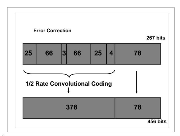
The final error correction step is to add the convolutional coding to the type 1 bits and all the other correction already added. None of this is applied to the type II bits, which have the 'make it if you can' protection applied! We are left with an output of 456 bits.
