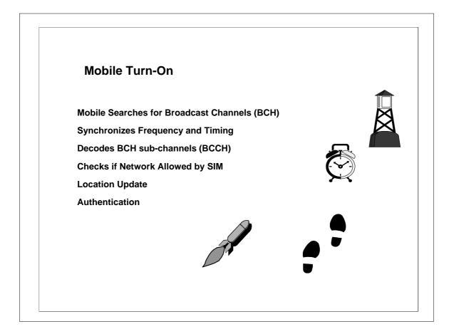
When a mobile first turns on, it searches all 124 channels in the downlink for signals. It will then order the channels by received signal strengths and check to determine if the channel was a BCH (Broadcast CHannel).
