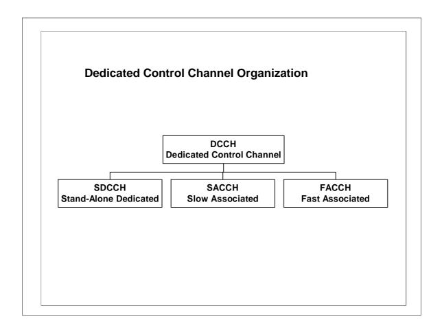
The Dedicated Control Channel (DCCH) is the only part of the Control Channel used during calls and call set up. We mentioned earlier that the mobile does not look at the CCCH during calls, it does however look at the DCCH. Remember that another way of describing a mobile on a call is it is in Dedicated Mode. This may be on the same frequency as the BCH, TCH or another altogether depending on how the system is configured.
