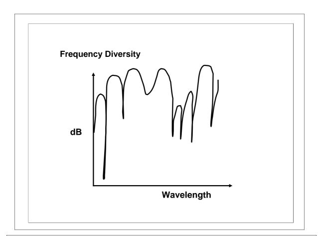
If there is an area that has bad multipath, such as urban areas with lots of reflections from buildings, the cell may have many fades. A fade is where the multipath signals destructively adds and produce a low level signal. The graph above shows these fades as a function of wavelength. If a mobile moves into a fade it can drop a call. There are two ways to avoid this problem:
