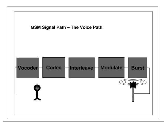
Now that we know how all the information is passed over the air-interface, we need to understand how the mobile and base station take a voice signal and get the data onto the bursts. This is the GSM Signal Path.
