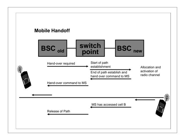
We have covered mobile power on and call establishment, but there is one other important area. During a call the mobile may have to change base stations. If the call is between faces of the same base station, this is performed locally. The case shown here is that where the base station is not the same.
