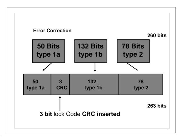
What does this error correction look like? The first step is to add the Cyclic Redundancy Check to the 50 type 1a bits. This is a three-bit parity code or checksum. At this point the 132 1b and 78 type II bits are not changed.
